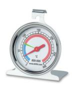
This stainless steel oven thermometer features a clear  $\varnothing 55$  mm dial with colour-coded zones. The green marker indicates the minimum temperature that commercial hot food display units should be kept at. The oven thermometer indicates temperature over the range of 0 to 300 °C in 10 °C divisions. The case measures  $43 \times 66 \times 80$  mm.
